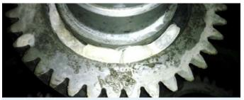
Gears with residue before trial
