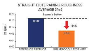
1. Roughness measurements in straight flute reaming on aluminum alloy (AISi7Mg)
