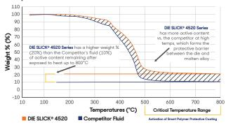
TGA is used to evaluate the thermodynamic stability of the active content (non-water material) of a die lubricant. This is a measurement of how much heat a lubricant can tolerate before decomposition, which is graphed as weight percent versus temperature.
