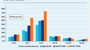
TOOL-LIFE RESULTS FOR ALL SIX MILLING CUTTERS USED TO MAKE THE COMPONENT
