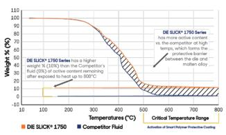
TGA is used to evaluate the thermodynamic stability of the active content (non-water material) of a die lubricant. This is a measurement of how much heat a lubricant can tolerate before decomposition, which is graphed as weight percent versus temperature.
