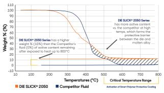
TGA is used to evaluate the thermodynamic stability of the active content (non-water material) of a die lubricant. This is a measurement of how much heat a lubricant can tolerate before decomposition, which is graphed as weight percent versus temperature.
