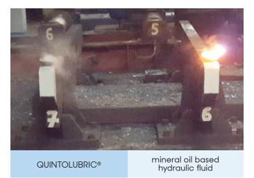
After **53 seconds QUINTOLUBRIC® self-extinguishes** and **stops burning**. The mineral oil based hydraulic fluid continues to burn.
