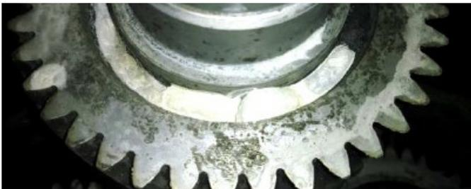
Gears with residue before trial
