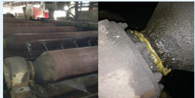
QUAKERTEK™ UX 4615-EP did not melt and remained at the application point on the roll neck
