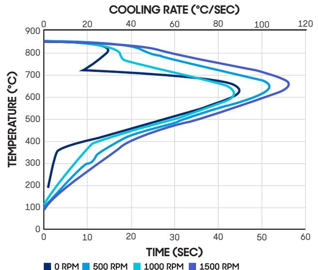
Figure 12 - The effect of agitation on the quenching characteristics of a normal speed oil.
