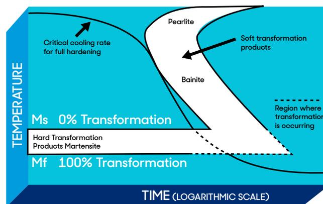
Figure 4 - A Time-Temperature-Transformation diagram illustrating the critical cooling rate for complete martensitic transformation.
