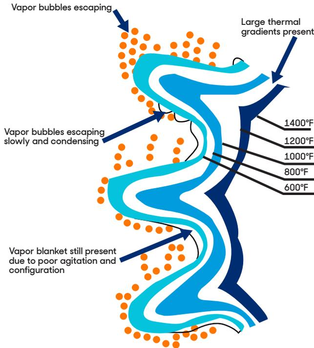
Figure 11 - Creation of non-uniform quenching by inadequate agitation.
