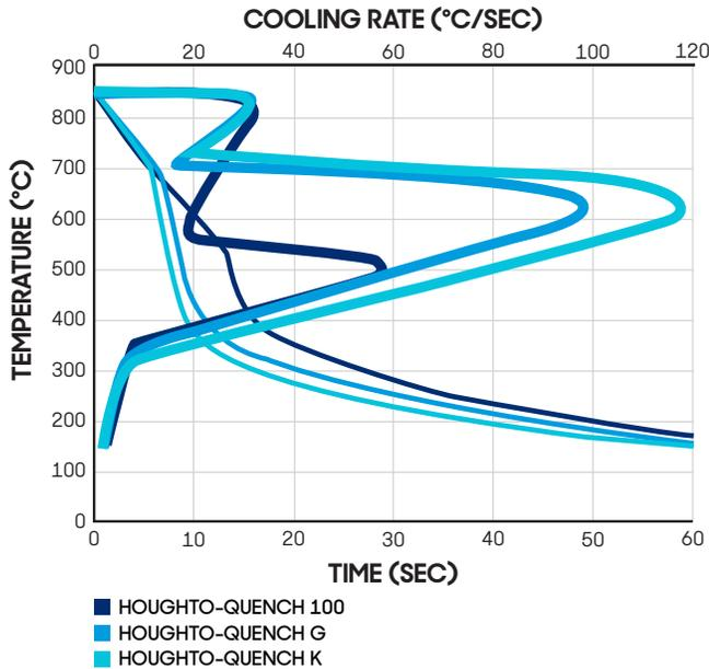
Figure 8 - Comparison of fast, normal and slow quench oils.
