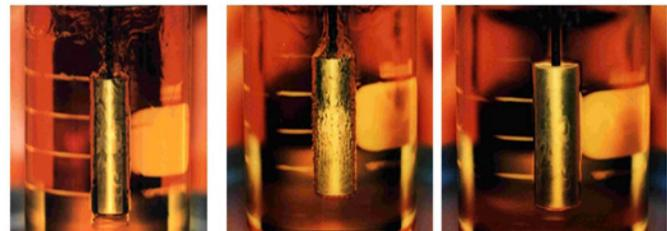
Vapor Blanket Stage      Boiling phase      Convection stage
