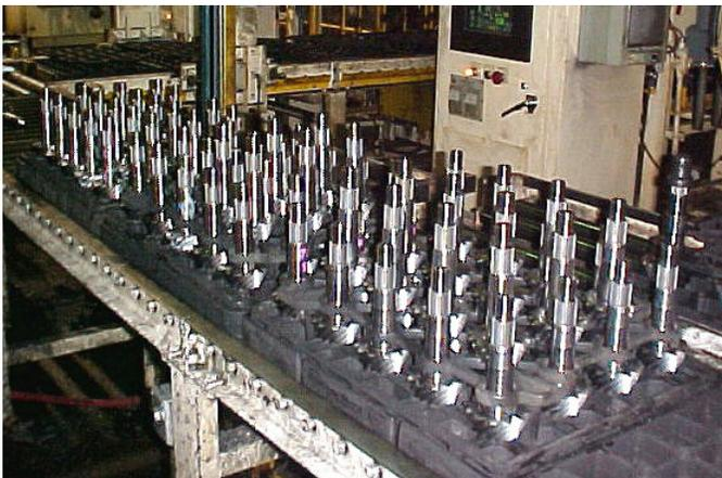
Figure 16 - Racking of pinions to minimize distortion.
