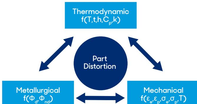
Figure 20 - Interaction of variables occurring during modeling of part distortion.
