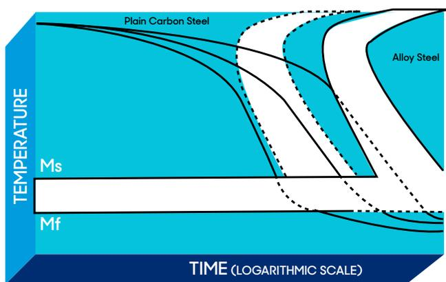
Figure 6 - The effect of alloy content on steel hardenability.
