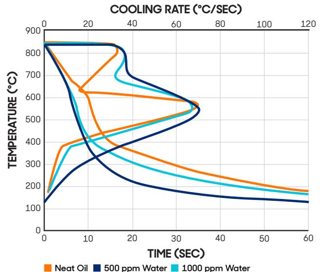
Figure 17 - The effect of water on the characteristics of a normal speed quenching oil.
