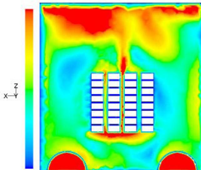
Figure 19 - Results of a CFD analysis of a quench tank, showing variations in agitation.
