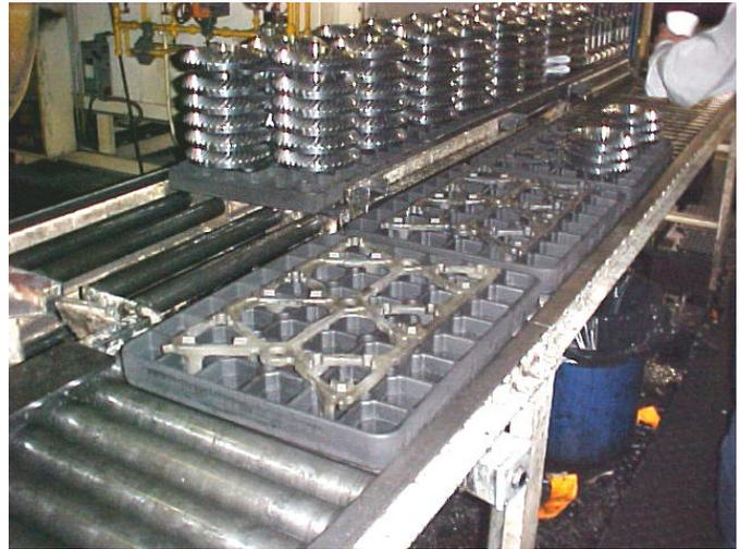
Figure 14 - Typical racking of gears on a grid prior to quenching.
