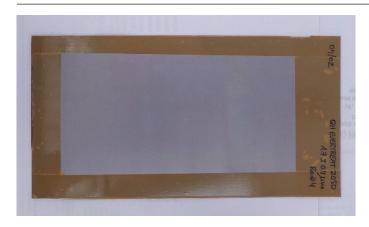
No corrosion observed on panel coated with QH EVERTREAT  $^{\rm m}$  2050 (DFT 1.5  $\mu m)$  after 8 hours of 5% NaCl at 35°C, 1.2 bar pressurized
