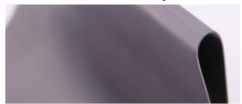
No adhesion loss in bending test: 3 mm cylindrical mandrel followed by tape adhesion test (ISO 1519)
