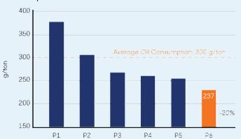
Setup Options: A series of different setups (P1 through P6) were necessary to best optimize the parameters of the QH FLUIDCONTROL™ MIDAS (oil concentration vs. speed and steel types, flow, pressure, etc.) and finally reach a 20% reduction in oil consumption.
