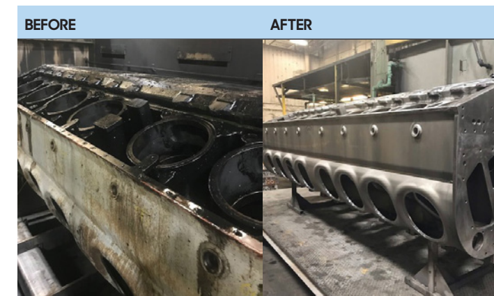
Large engine block cleaned with HOUGHTO-STRIP®
