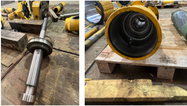
The bonnets were in nearly new condition after being cold stacked with STACK GUARD™ for seven years
