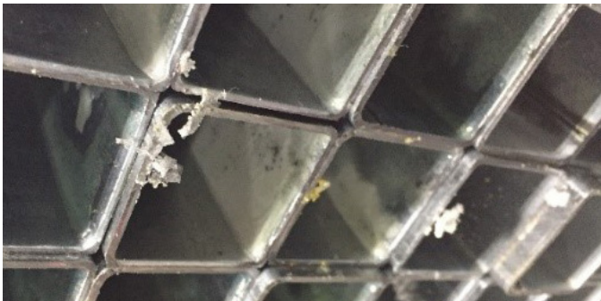
Tubes with competitive coating: Coating was seen peeling off during storage.
