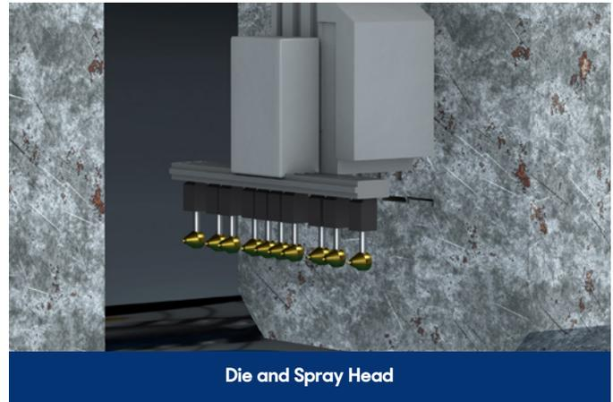
Proper preheat is also critical to minimize thermal shock during start-up. During the start-up process, a start-up lubricant or die conditioner should be used instead of a conventional die lubricant. These oil- and wax-based products allow for sufficient release of the parts while the die gets to operating temperature.
