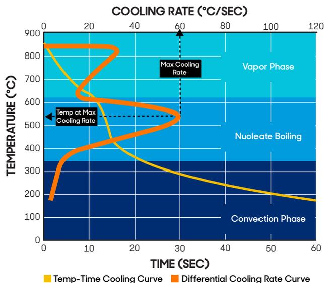
Figure 7 - Temperature-time cooling curve and the differential cooling rate curve.
