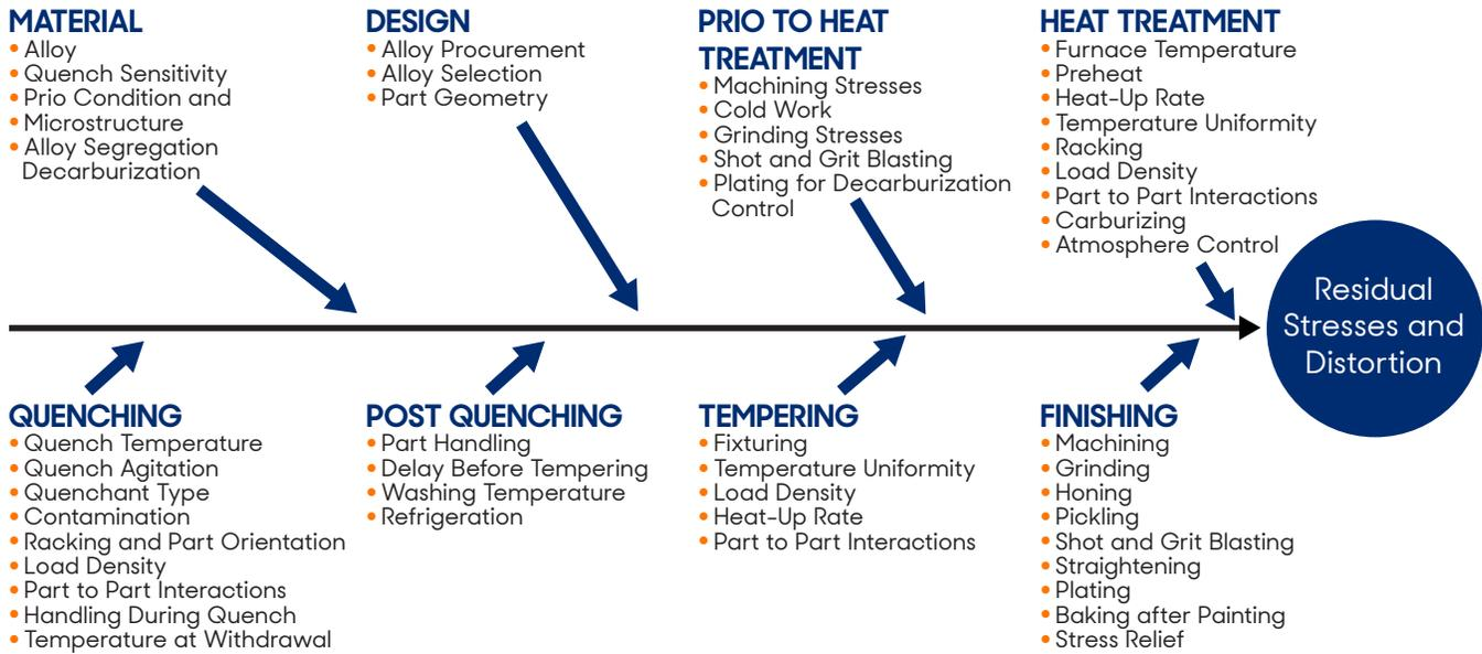
Figure 10 - Fishbone diagram of the potential causes of residual stresses and distortion.
