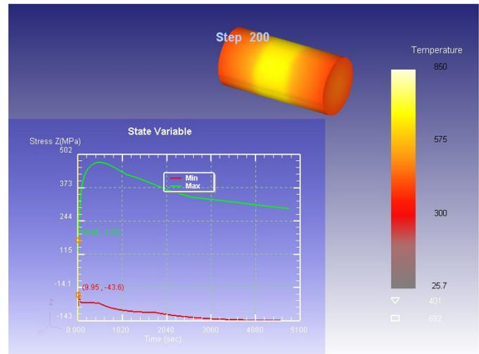
Figure 21 - Simple geometry modeled, showing the development of residual stresses.
