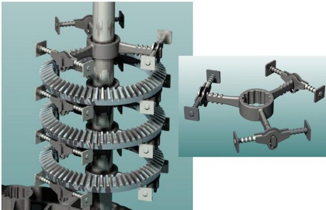
Figure 15 - Example illustrating proper racking design to minimize distortion.
