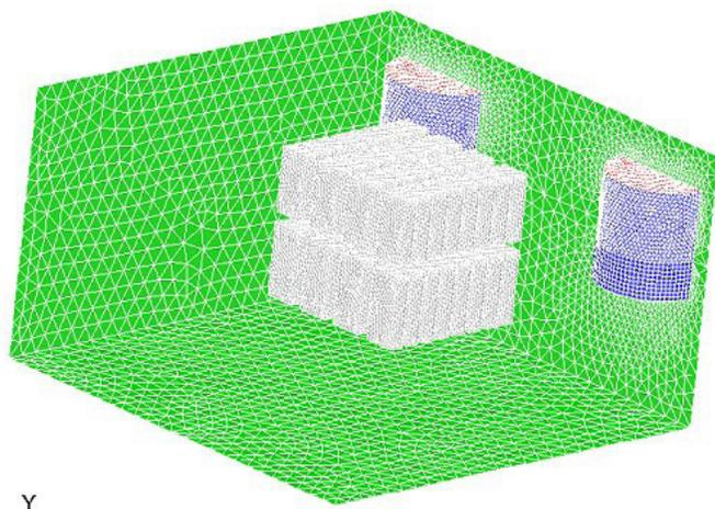
Figure 18 - Example of a meshed grid in a hypothetical quench tank.
