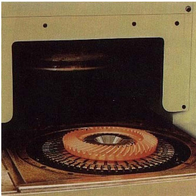
Figure 13 - Press quenching of an automotive ring gear.
