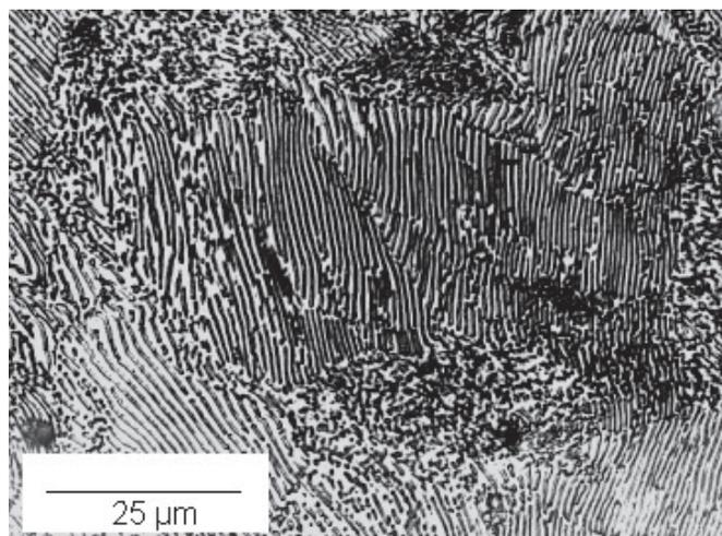
Figure 5 - Pearlite resulting from slowly quenched high-carbon steel.
