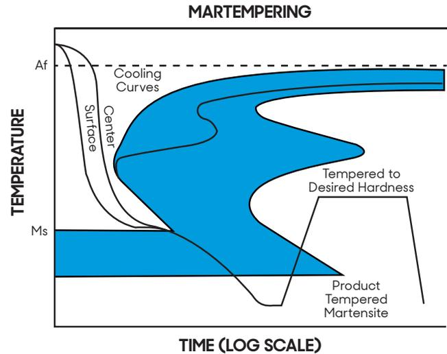
Figure 9 - Schematic of mar-quenching to minimize distortion [1].
